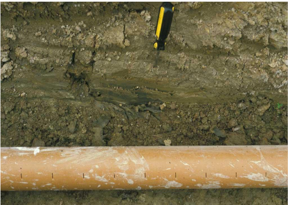
Figure 12-3: Grey, low permeability subsoil. Note grey colour and 'plasticine-like' nature of the subsoil. (Photo: Donal Daly)
