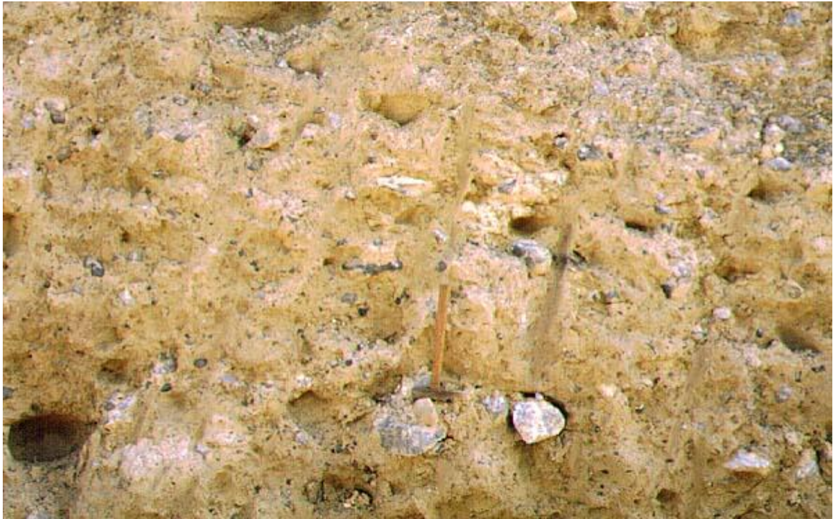
Figure 21-4: Moderate permeability, free-drained subsoil (glacial till (sometimes called 'boulder clay')). Note brown tinge to an originally grey material (grey as it is a limestone till), indicating oxidation and unsaturated conditions. (Photo: Donal Daly)
